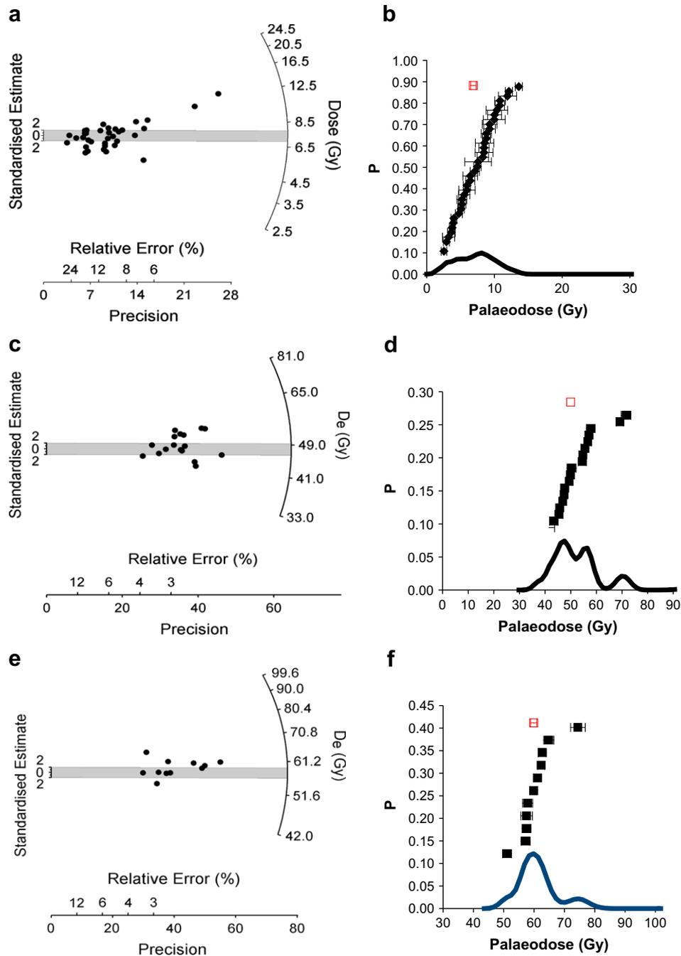
**Fig. 5.**  $D_e$  distributions for samples Hi2006II (a, b), Hi2006VI (c, d) and Hi2006I (e, f). Showing radial plots on the left and probability (P) density plots on the right with individual aliquot  $D_e$  plotted above (closed square) and the arithmetic mean of the data (open square).
