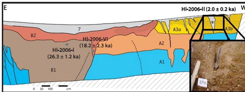
Fig. 2. Western part of the Gerdab trench logs on the Dehshir fault with the position and the dates of the OSL samples. Sedimentary units are indicated by different colours and labelled numerically. Units A and B are young alluvial and colluvial units. Unit 7 denotes the sandy silty unit infilling open fissures and mantling the ground surface after occurrence of the last surface rupturing earthquake. Inset shows where Hi2006II sample was collected.
