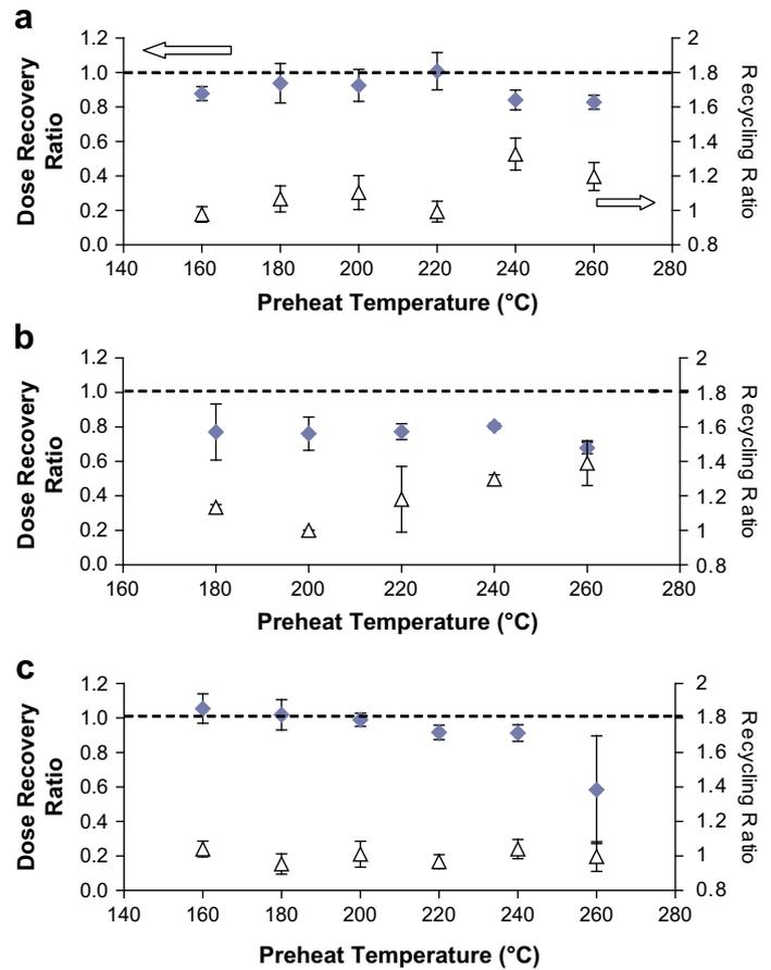
Fig. 3. Recycling ratio (open triangles) and preheat plateau for dose recovery test (solid diamonds) using different preheat temperatures and heating rates. (a) Heating rate of 2 °C/s for sample Hi2006II; (b) heating rate of 5 °C/s for sample Hi2006II and (c) heating rate of 2 °C/s for sample Hi2006VI. Note: dashed line denotes the given laboratory dose.
