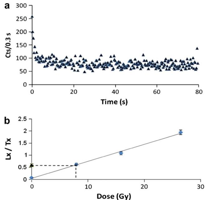
Fig. 4. An example of the OSL decay and SAR growth curve for sample Hi2006II showing (a) the weak natural OSL signal and (b) despite this, a good SAR growth curve could be measured.
